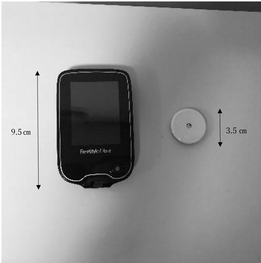
Fig. 3 A reading device and a disposable sensor of the FreeStyle Libre Flash glucose monitoring system.
